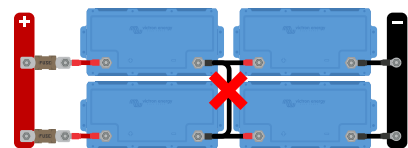
Do not interconnect midpoints nor connect anything else at the midpoints
